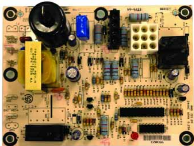
Figure 25: Ignition Control Board
